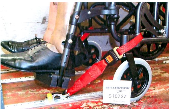
Fitting the front restraint
